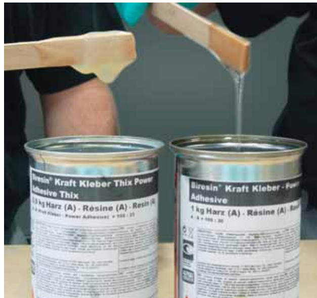
The thixotropy of Biresin® Power Adhesive Thix (left half of picture) is much higher than its predecessor.
