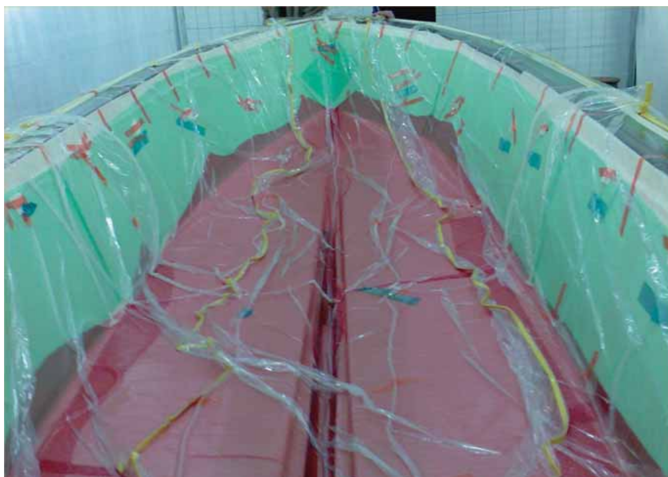
Production of CRP boat hull with infusion process
