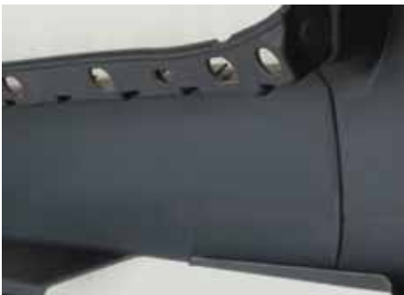
Low-pressure RIM mould made of SikaBlock® M940 and the associated sillboard panel made of Biresin® RG53
