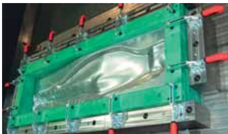
Incremental forming of a gear-box console (metal sheet made of DC04 with a thickness of 1.2 mm)
