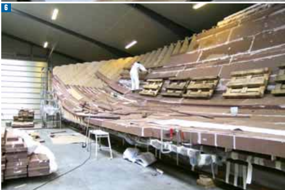
4 The mould for a superstructure side panel for the Royal Denship 105 awaits final grinding and polishing. 5 The 30kW milling head on the small CNC machining centre can cut aluminium, epoxy and carbonfibre panels, as well as polyurethane paste. 6 The portside of the Royal Denship 105 mould substructure is pieced together in preparation for PU foam to be applied. Once that is rough milled, it will be coated in PU paste for fine milling.
